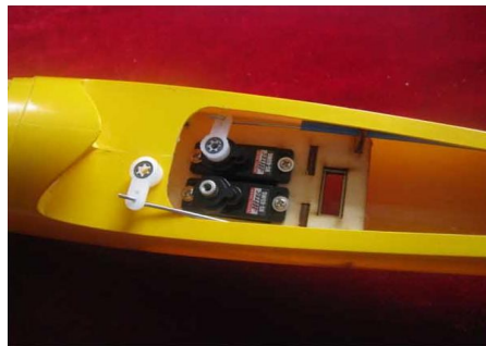
4. Use Adhesive Tape to confirm the location of Servo Horn, in order to make sure the Angle of Elevator is correct.
