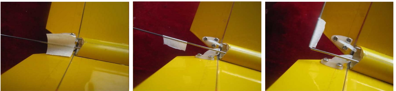
5. Bend Push Rod in 90 Degree and connect Servo Horn.
