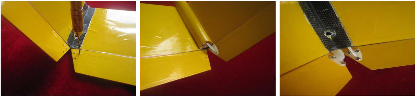
3. Connecting Push Rod and Servo Arm.
