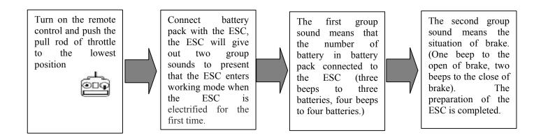
Remark: if the motor suddenly stops when your model airplane are flying, you shall immediately push the pull rod of throttle to the lowest position and then push to the high position. Then the motor will restart. You
